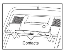
not display your heart rate accurately. Before using the handgrip pulse sensor, remove the clear plastic film from the metal contacts. In addition, make sure that your hands are clean.
